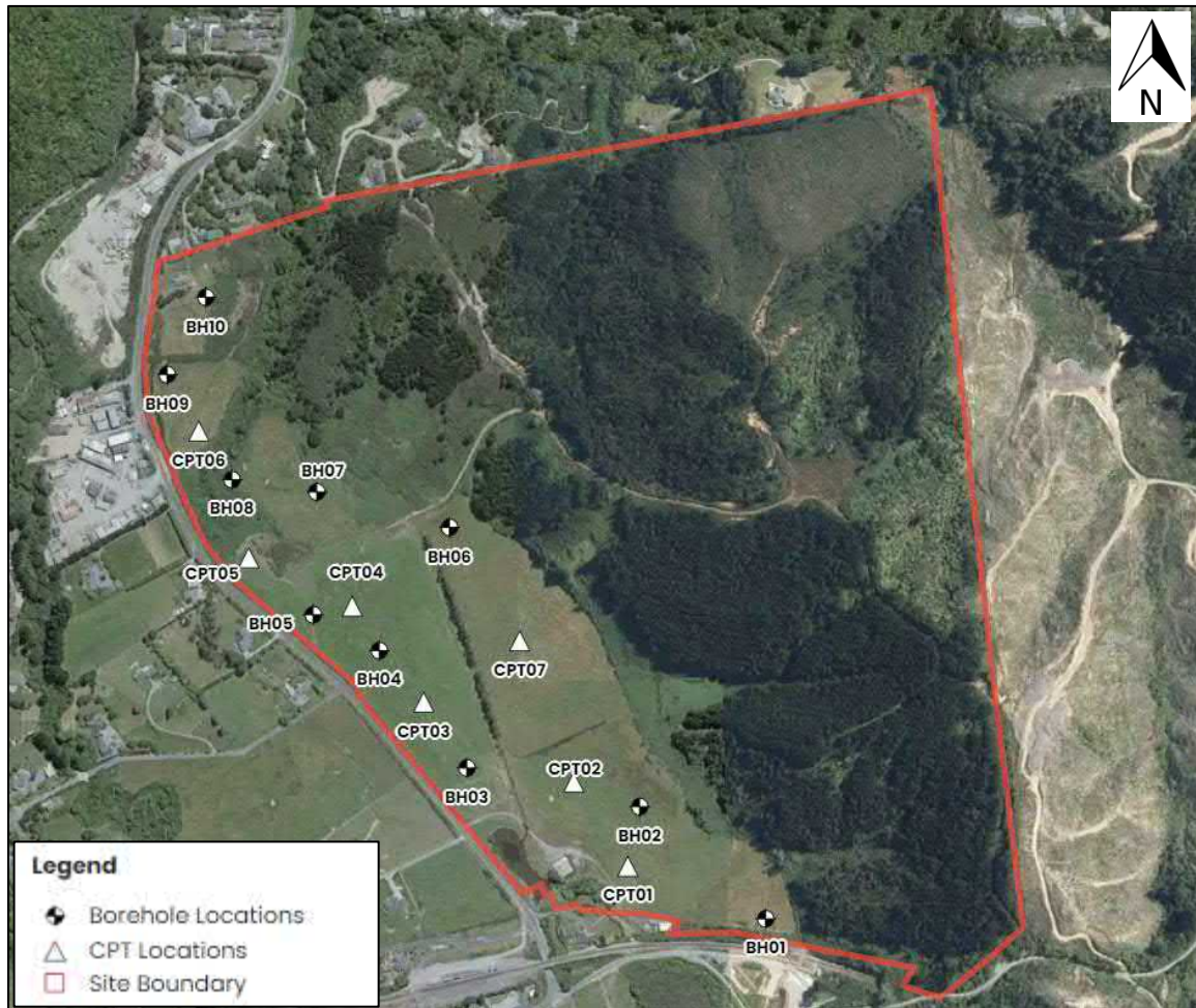
Figure 7: Subsurface Investigation Locations
