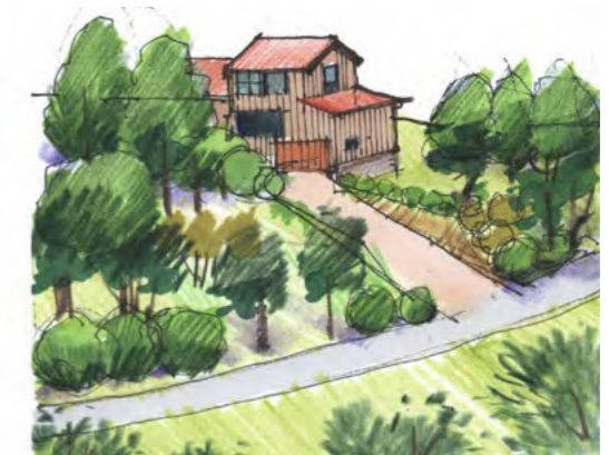
✗ Driveway runs straight up the contour necessitating earthworks.
