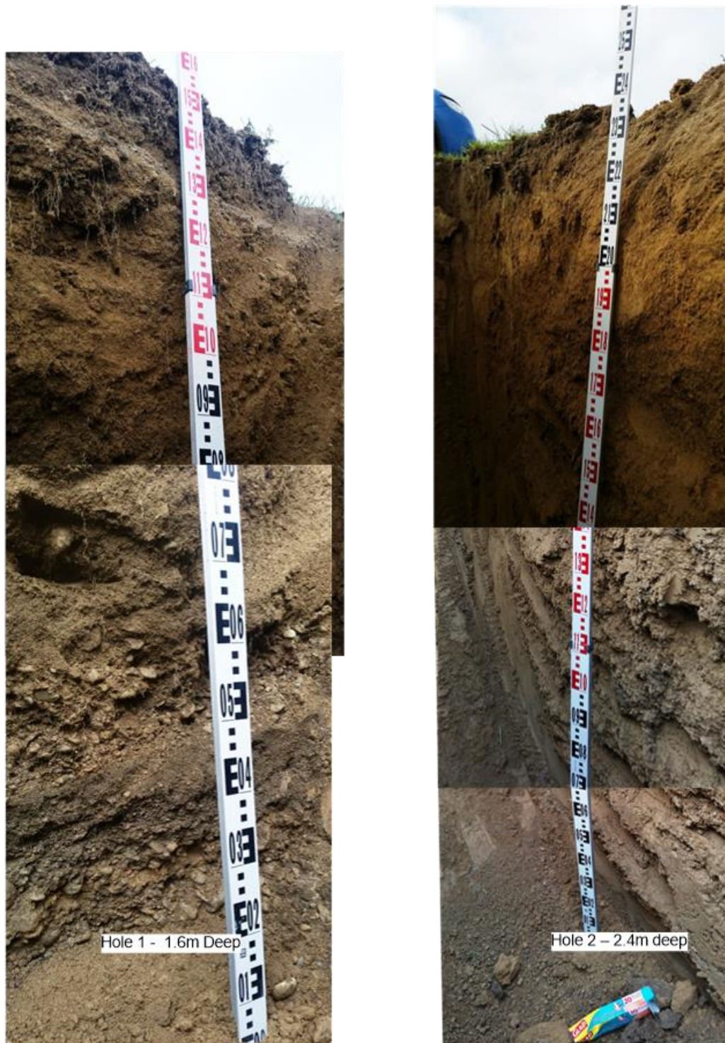
Figure 8. Test pits in the northern end of the proposed subdivision site on the alluvial flats. Soil profiles were consistent with the GIS database soils and geological descriptions and provided 0.8-1.2m of a medium brown silt loam topsoil/ surface layer, underlain by relatively free draining alluvium. The soil moisture content was relatively low compared to field capacity, despite the samples having been taken mid-winter with moderate antecedent rainfall.
