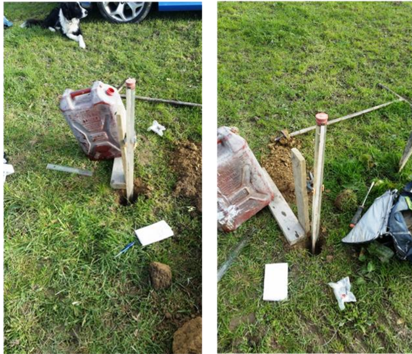
Figure 21. Constant head infiltration tests near the surface; (300 and 450mm depth), as per NZS 1547:2012.
