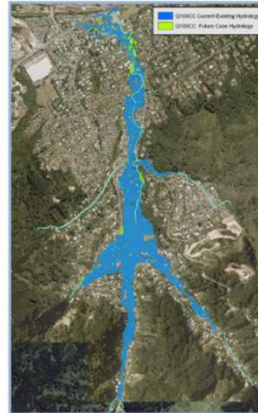
Figure 19 Current Existing vs. Future Case Comparison of Predicted Flooding Extents in the Q 100 with Climate Change.
