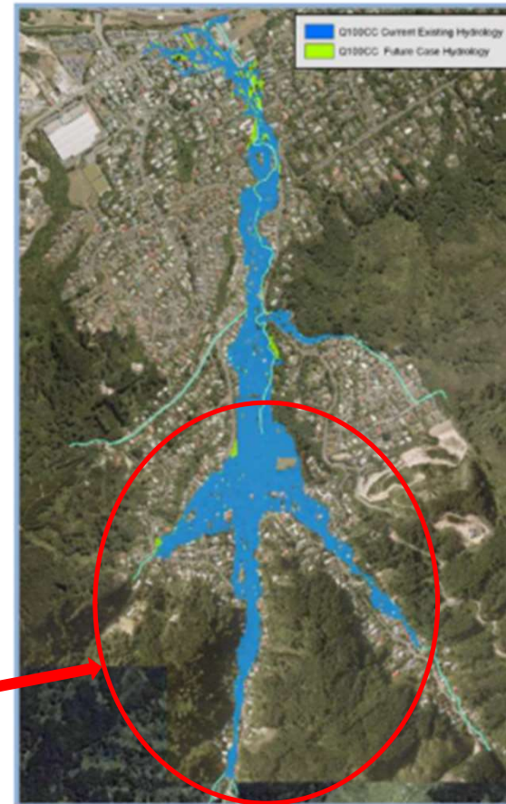
■ Figure 19 Current Existing vs. Future Case Compare the Q 100 with Climate Change.
