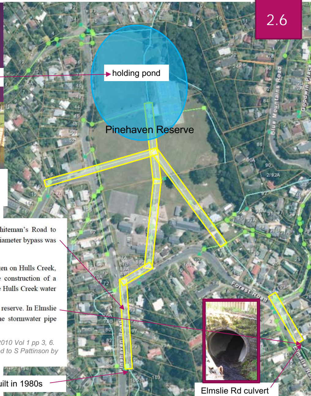
Combined drain discharges to open stream & ponding area in Pinehaven Reserve
