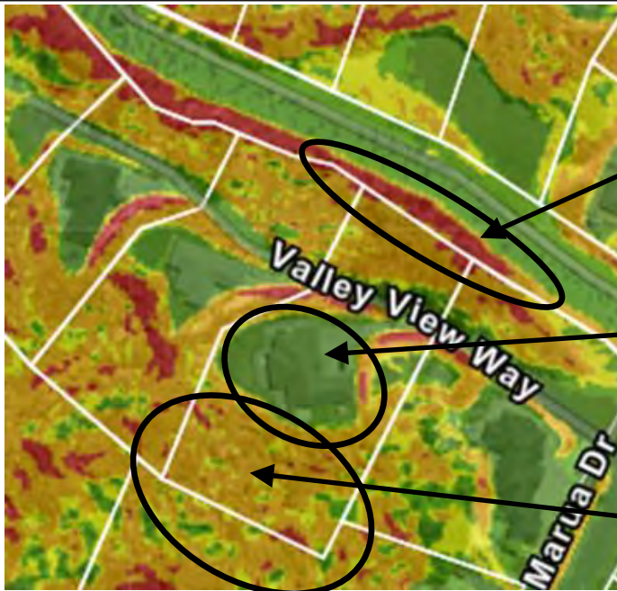
Fig.1 Areas of incorrect or inconsistent High Slope Hazard rating at 3 Valley View Way
