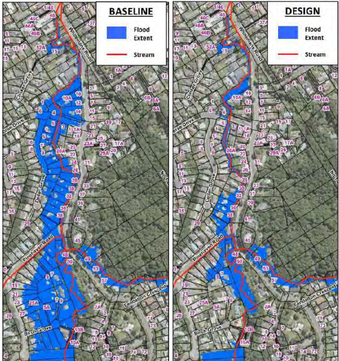
Figure 7: Modelled extent of flooding during the 1-in-100-year event for the baseline/current scenario (left) and design scenario (right) (from the Updated FHA dated 15 June 2020)
