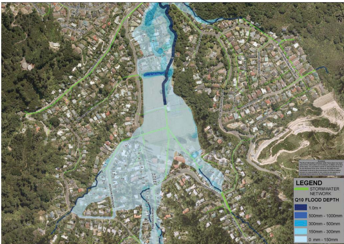
Figure 4.1 – Base scenario Q10 flood inundation
