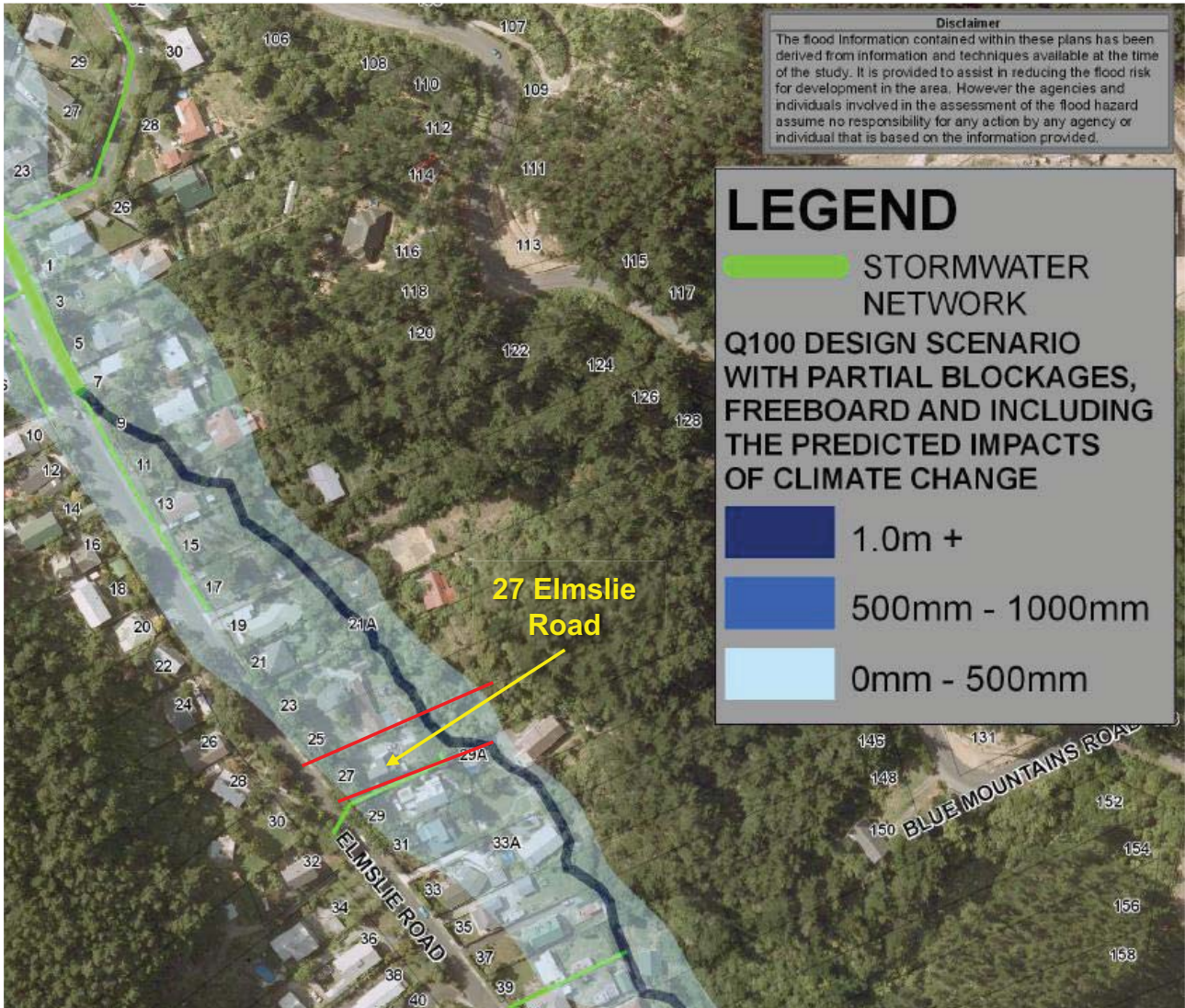
Figure 5.1 – Q100 (including culvert blockage, climate change and freeboard) flood extent at 27 Elmslie Road
