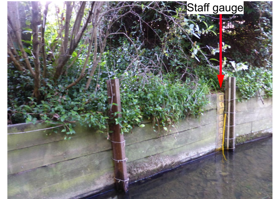
3 - Staff Gauge on True Right Bank approx 3.4m upstream from Footbridge Weir
