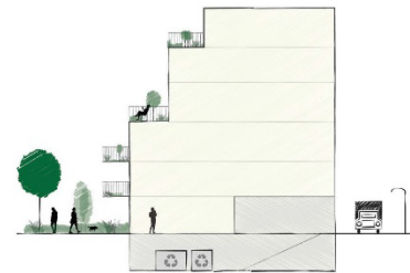
DIAGRAM 5 - SERVICE AND DELIVERY AREAS FOR MIXED USE PREFERABLY LOCATED AWAY FROM PEOPLE ORIENTED AREAS
