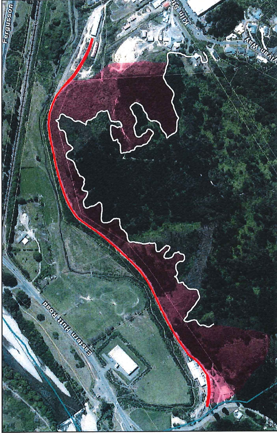
Figure E1: The purple shaded area represents the area of Silverstream Spur that is not recommended for residential development, in terms of noise from the Silverstream Railway locomotive 509 activities. (Base Image: UHCC GIS).
