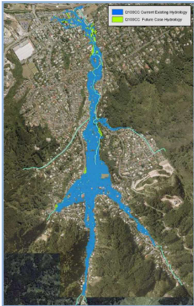
■ Figure 19 Current Existing vs. Future Case Compar the Q 100 with Climate Change.
