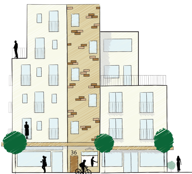
DIAGRAM 11 - VARIATION IN COLOURS, SCALE, PLACEMENT OF WINDOWS, ROOFLINES ETC CAN ENHANCE VISUAL INTEREST
