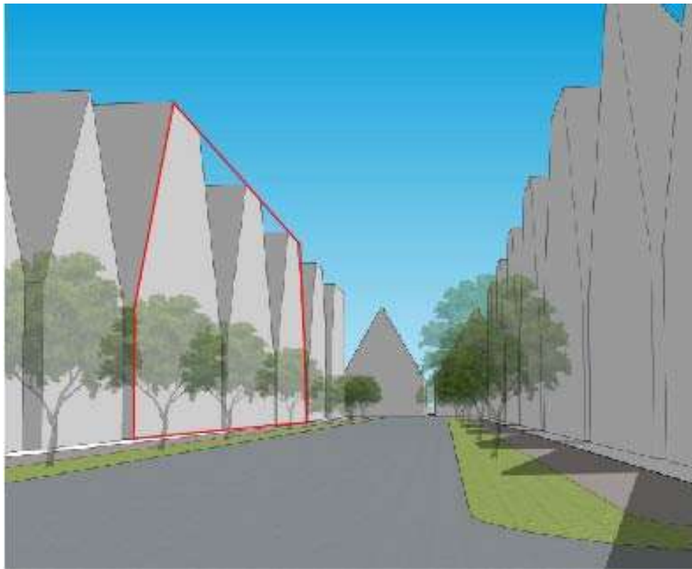
Figure 7 - An example of the bulk envelope (red line) of a site that is the result of amalgamating three sites, based on Attachment D, SK04 where the maximum height is not controlled by the HIRB (20m) and no internal HIRB control is applied.
