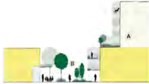
DIAGRAM 10 - GROUND FLOORS DESIGNED TO SUPPORT A HUMAN SCALE AT STREET LEVEL
