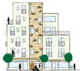
DIAGRAM 1 - VARIATION IN COLOUR, SCALE, PLACEMENT OF WINDOWS, BALCONIES ETC CAN ENHANCE VISUAL INTEREST
